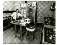
pling uses Cartridge Control Corp.'s high speed (120 inches second) master duplicator capable of handling 8-track, cassette and open reel tapes.
