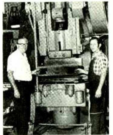
DOC ULRICH, plant manager (left) and an employee hold a piece of metal formed in the 110-ton punch press behind them. The huge machine, part of a complete metal working section, costs $30,000.
