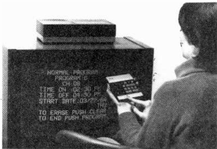
RCA introduces a remote programmable VCR with the Convertible VCP900. The unit uses a microcomputer chip that allows user to set the clock remotely and pre-program up to eight programs a full year in advance. Alphanumeric graphics appear on the tv screen, simplifying the programming process.
