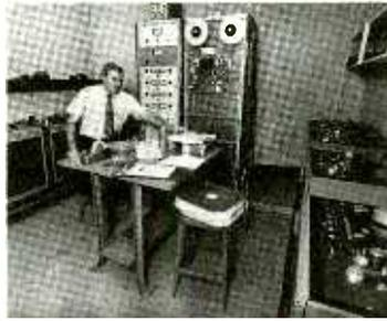
CHIEF AUDIO engineer Jerry Applying uses Cartridge Control Corp.'s high speed (120 inches per second) master duplicator capable of handling 8-track, cassette and open reel tapes.
